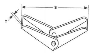
Toggle Wings are a four-piece fastener consisting of two matching steel wings, an internally threaded nut, and a wire spring providing the necessary tension to open and close the wings.
